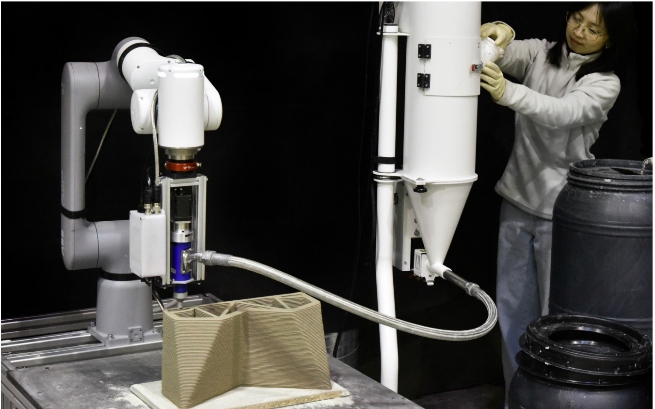
3D Printing Process in the laboratory conditions @Tizian Rein
