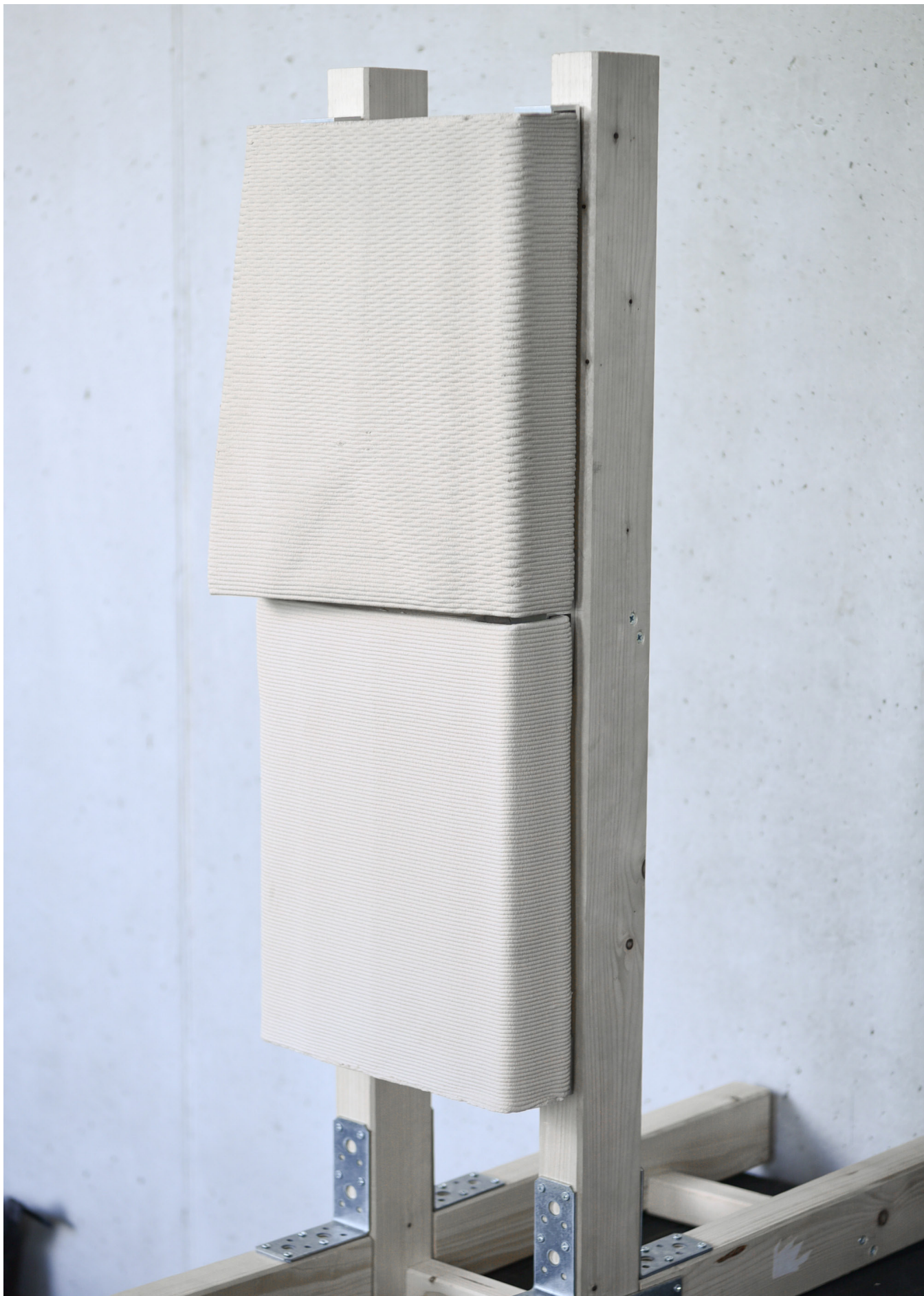
Mockup with the Fired Bat-Tile and one Regular-Tile in the Tonality Substructure 1:1
