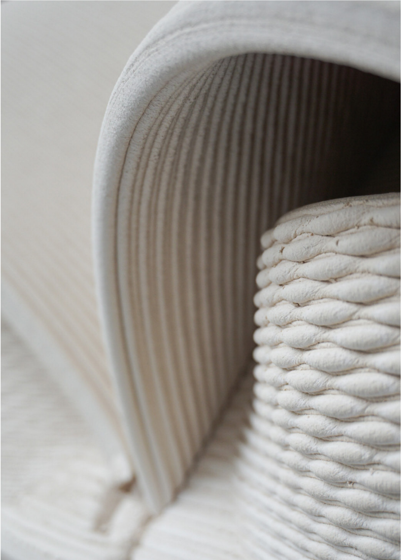
Nest opening and surface texture for grip - 1:1 Prototype
